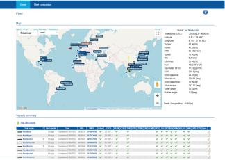
**SeaPerformer** system is an advanced solution for fleet management and ship operational performance. It collects data from subsystems and dedicated sensors and presents them both onboard and on the web application. A reliable analysis gives decision support to fleet manager and leads to reduction of operational costs and negative impact on the environment by fuel consumption optimisation.
