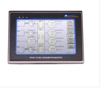
EFCM is designed to cooperate mutually with SEEMP Set giving a readable and detailed analysis of ships operations at sea. The range of Enamor ltd products is dedicated for ship-owners who want to find reliable solution to reduce ship energy consumption indicating the most effective ways to control fuel consumption and CO<sub>2</sub> emissions.
